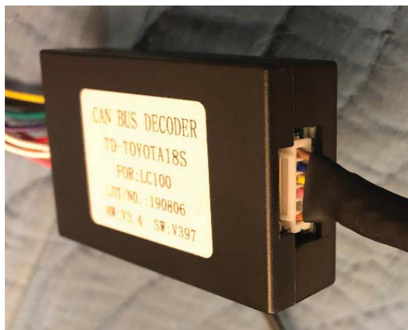
I= ZF-1301S Agreement Tie Line Harness: Side vent transfer case lock and airbag light. Flat 6 connector goes to CanBus module
