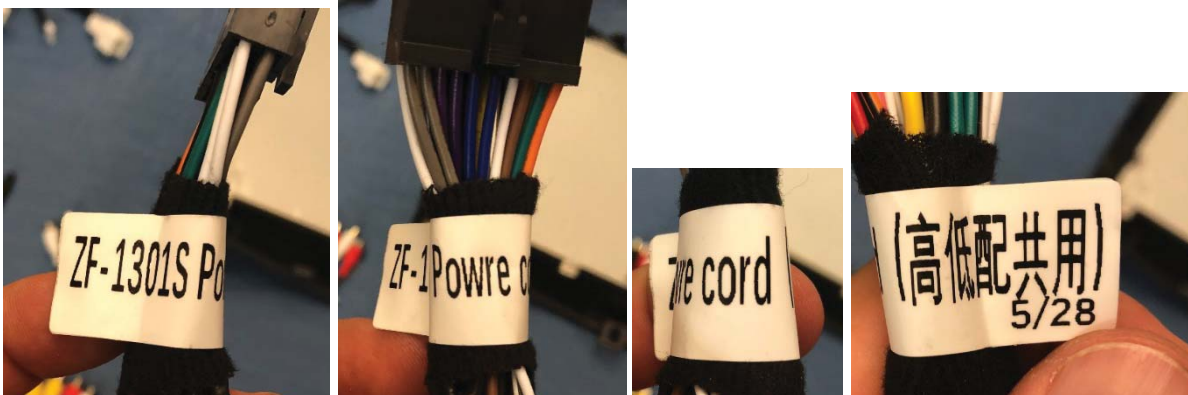
H= Main Radio Harness (Power Cord)
