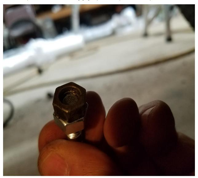
To install the new stud use the 12mm socket to engage with the factory nut and install the stud until the shoulder contacts the housing. At this point switch over to the 13mm deep socket and place it over the stud to engage with the 13mm DIN nut and further tighten the stud to release the DIN nut from the factory nut.
