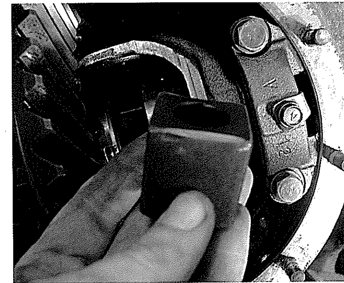
The spider piece after grinding.
