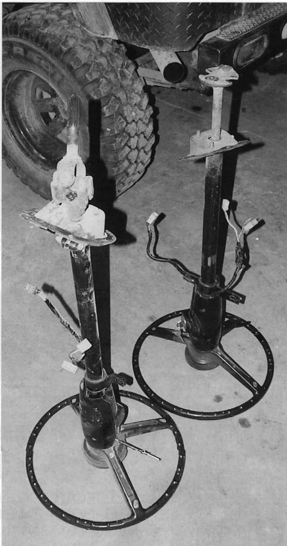
FJ40 (right) and FJ55 (left) steering columns before disassembly. The primary difference (the u-joint as opposed to the rag attachment) is clearly visible.
