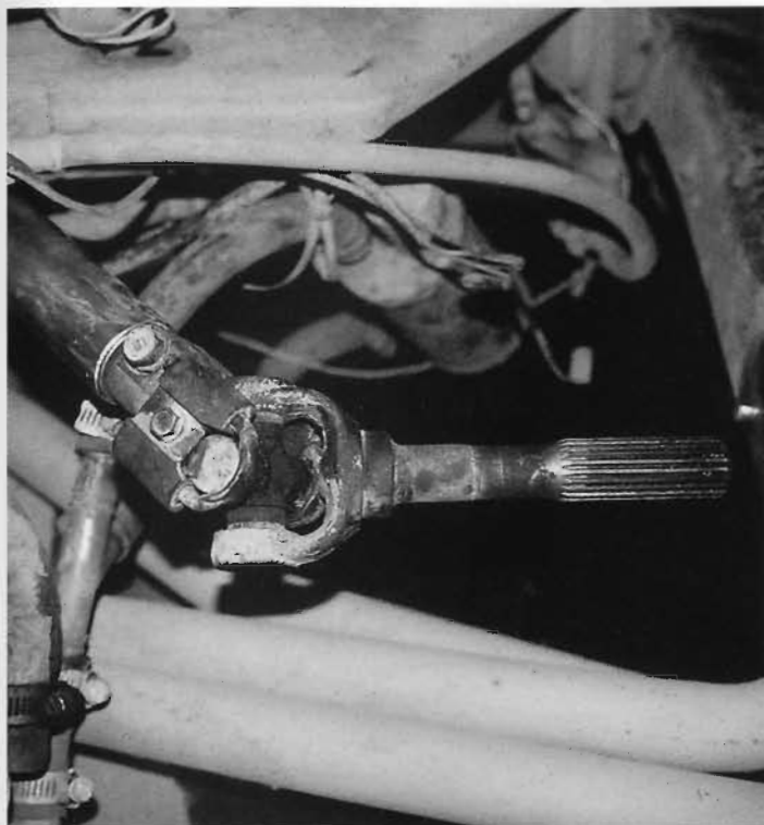
This is the factory FJ55 intermediate shaft attached to the modified steering column. The next step after this picture was taken was to lengthen the shaft to reach the steering box.
