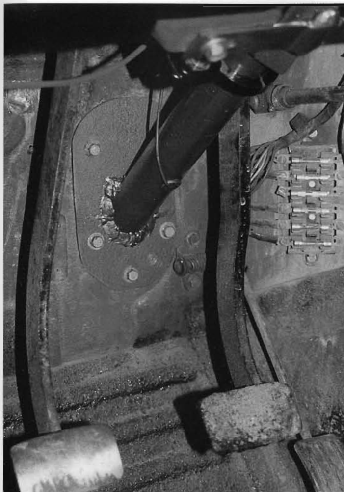
This is the plate which secures the steering column of this '68 FJ40 to the firewall.
