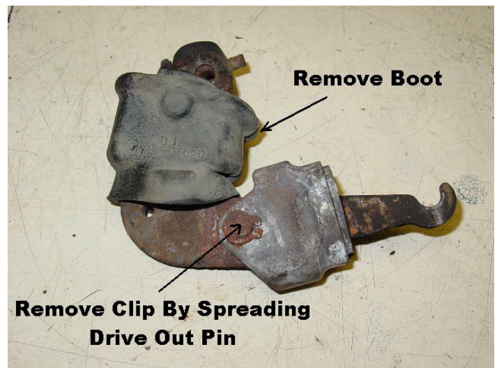
Fig. 8 Remove the boot
