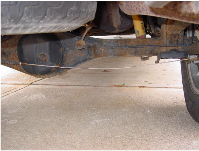
Fig. 1 Sagging park brake cable
