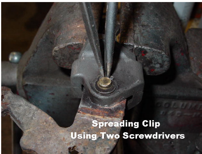
Fig. 9 Remove the U clip
