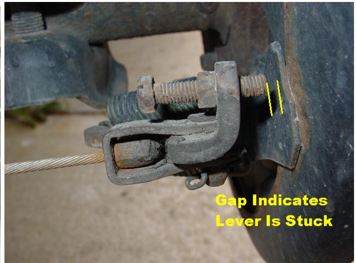
Fig. 2 Bellcrank stop off backing plate
