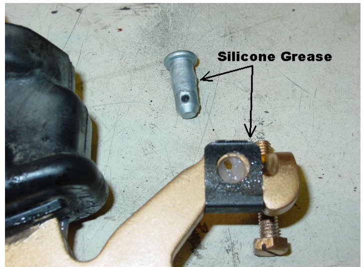
Fig, 14 Grease points
