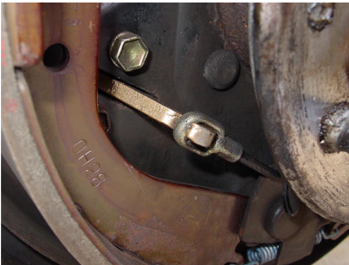
Fig. 16 Transfer cable must be attached
