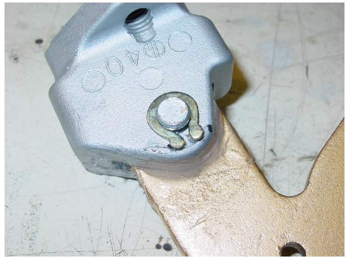
Fig. 13 Installing the lever and pin
