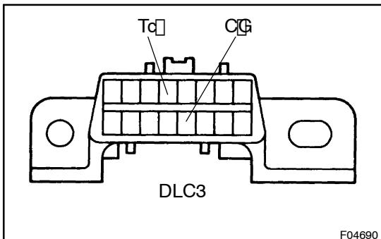
(6) Using SST, connect the terminal Tc to CG of DLC3.
