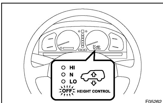
(7) Read the test DTC output by the height control OFF indicator light.
