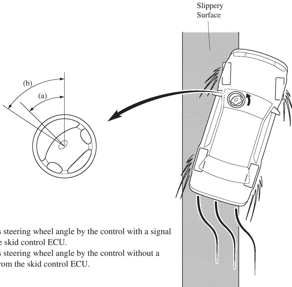
(a): Driver's steering wheel angle by the control with a signal from the skid control ECU.
