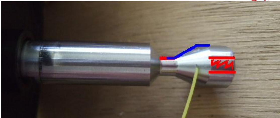
The narrow red section is cutout to allow the pin to be reinstalled without having to remove the pin follower pretensioner under the throttle linkage. This is a real plus as particularly in later models that have a throttle position sensor, access is a real pain...
