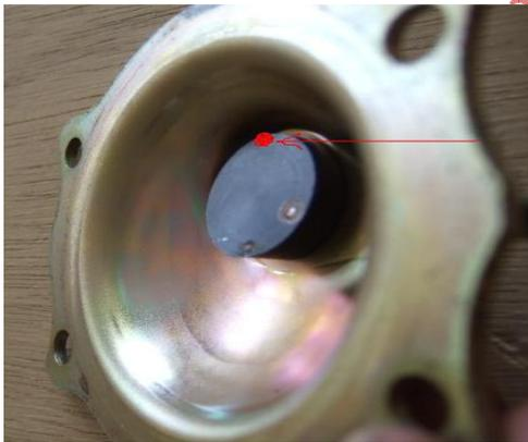
Grinding this plate is sometimes necessary to get the pin to rise high enough. This disk is normally rotated to allow more or less off boost fuel (usually more). This is not a problem now, we will have too much anyway.... So it is a redundant piece (mostly)
