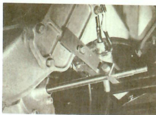
FIG. 32 - POSITION OF SHIFT YOKE SHAFT SUPPORTS.
