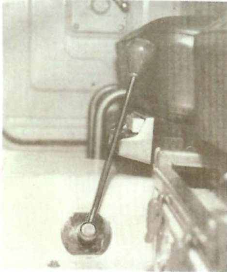
FIG. 25 - LOCATION OF THE INSTALLED TUNNEL PLATE SHIFTER AND BUSHING ASSEMBLY AND ALSO POSITION OF SHIFTER ROD WITH OVERDRIVE IN "DIRECT DRIVE".
