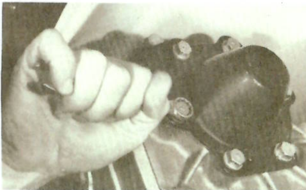
FIG. 3 — REMOVING THE SPLINE SHAFT CAP FROM THE TRANSFER CASE.
