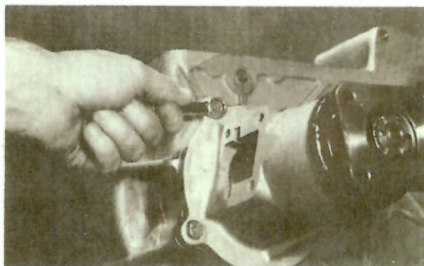
FIG. 8 — REMOVING THE FRONT DRIVE EXTENSION HOUSING FROM THE TRANSFER CASE.
