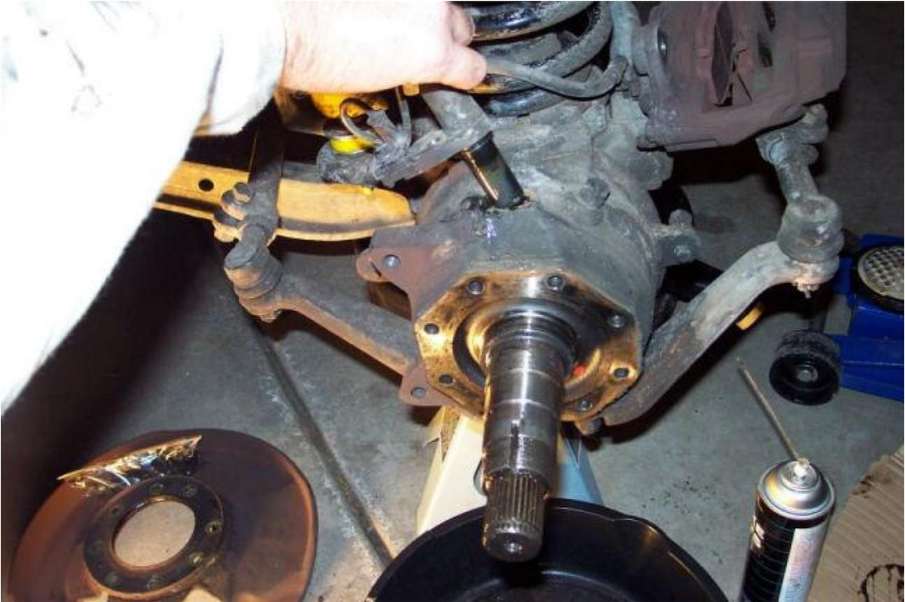
Using a brass bar and hammer, tap the knuckle spindle to free it from the knuckle.
