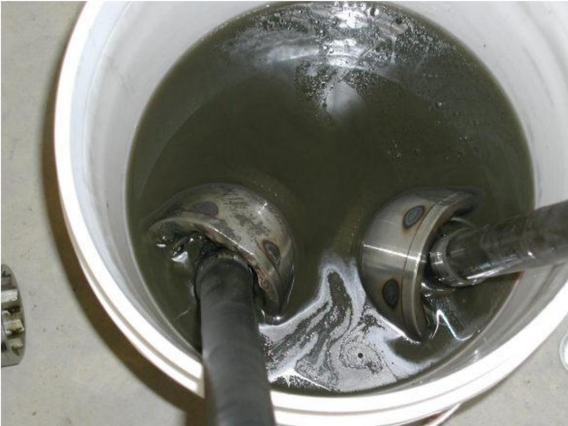
At this point some will dis-assemble the birf from the axle. A benefit to doing this is to swap sides. The birfs wear on one side and swapping sides extends the life in some cases.
