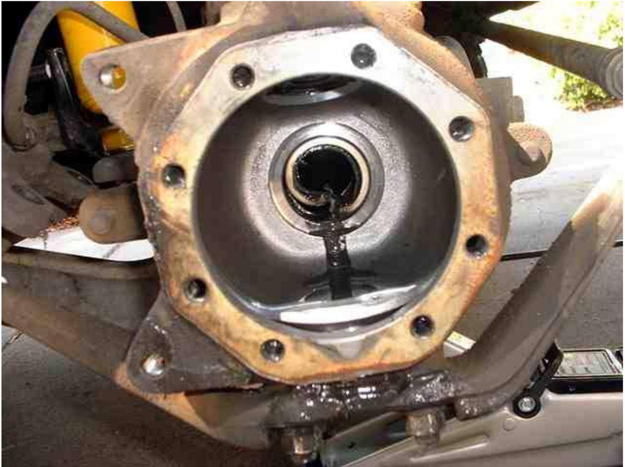
Shine a flashlight into the axle housing and look around. There should be nothing visible loose in the housing and there should be an index ring about 2 inches from the oil seal flush against the inner lip of the machined surface (it may look like part of the housing). This ring can occasionally come loose. If it has it will likely be lying in the housing and you will need to reseal it somehow (there are posts on this).
