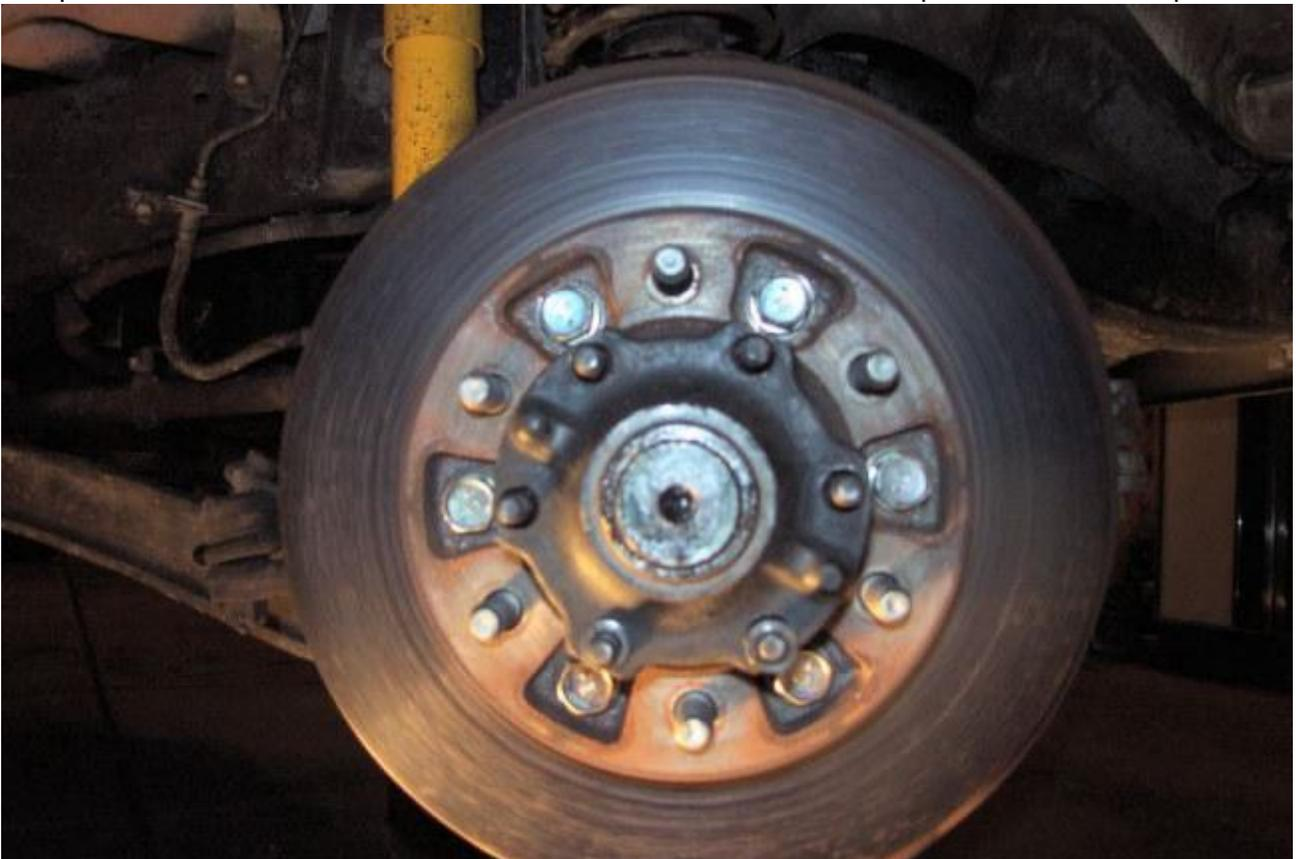
With the cone washers removed from the Flange, remove the Drive Plate.
