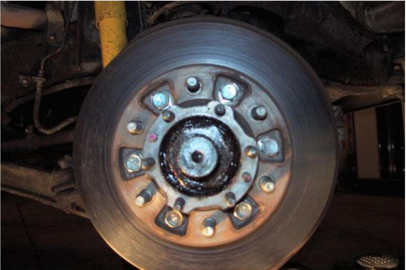
Next you will see a lock washer, use a screwdriver to remove this by bending the tabs to the middle position, even with the rest of the washer
