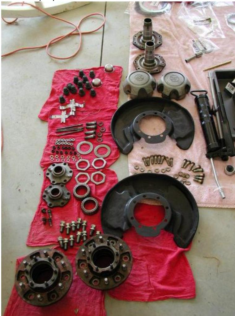
Install new studs in lower knuckle - Use Loctite
