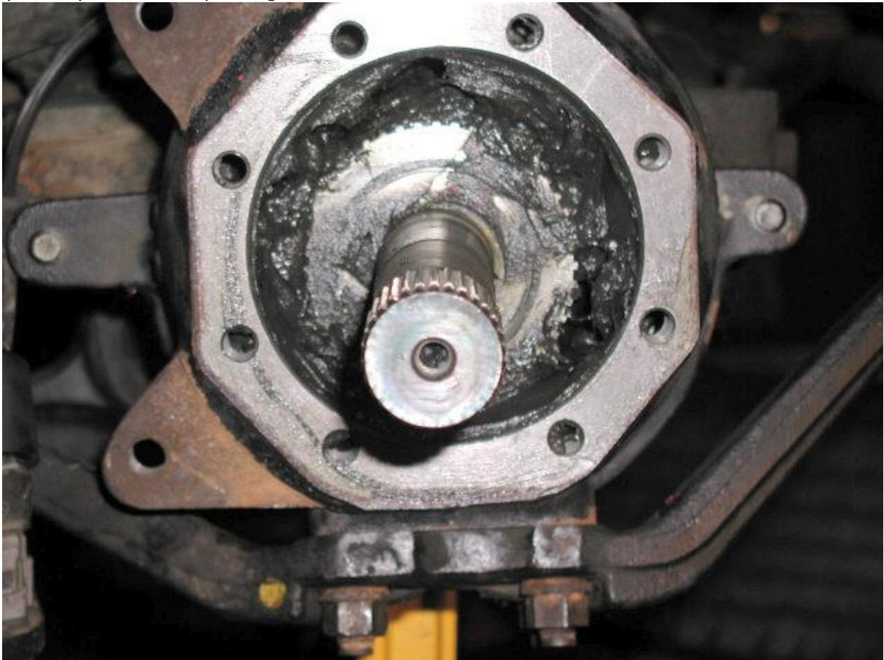
Install the 2- 10MM x 1.25' pitch studs in the knuckle to help with positioning the following items
