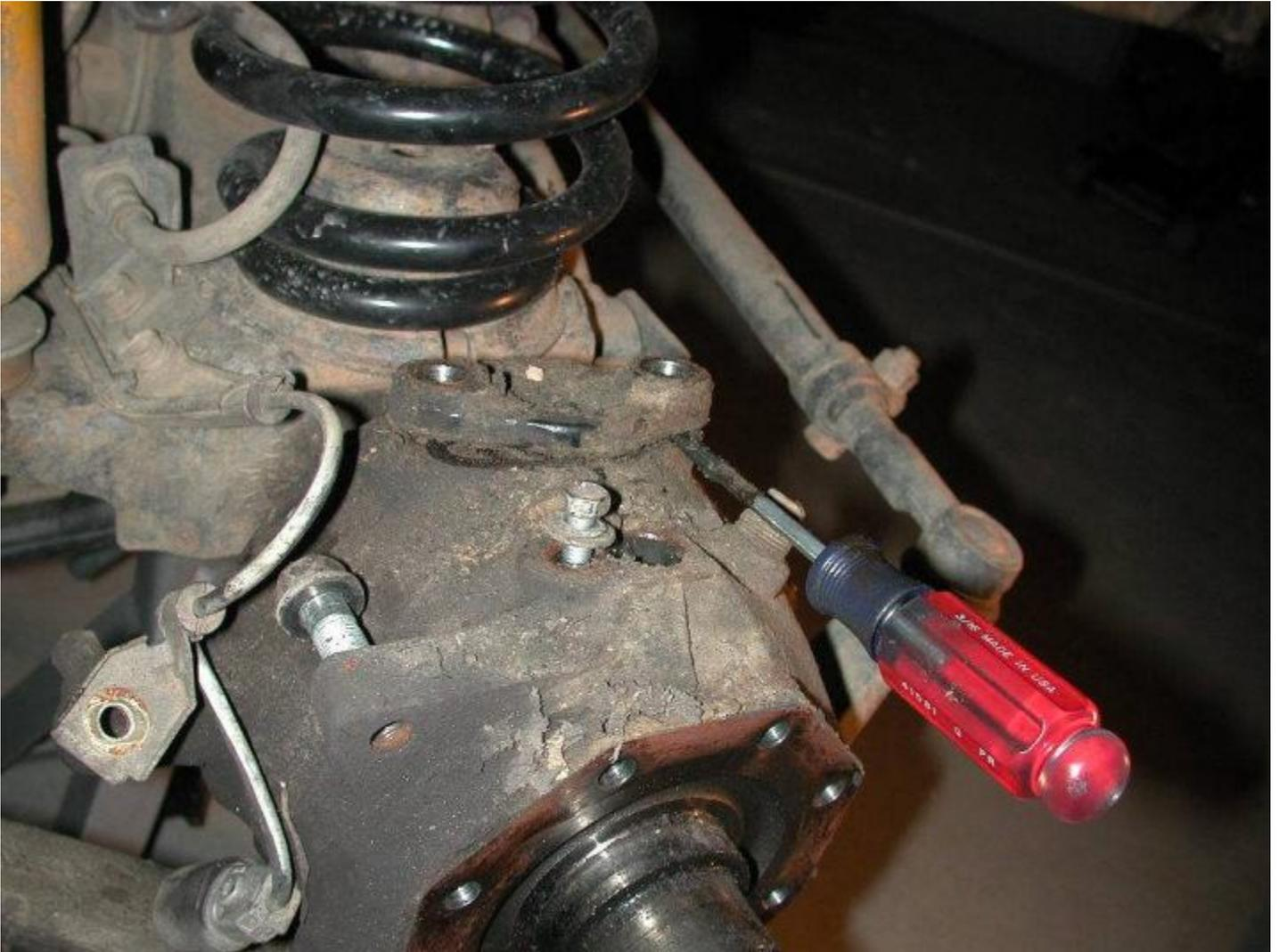
Loosen the 4 nuts (17MM) that attach the lower control arm/bearing housing to the knuckle
