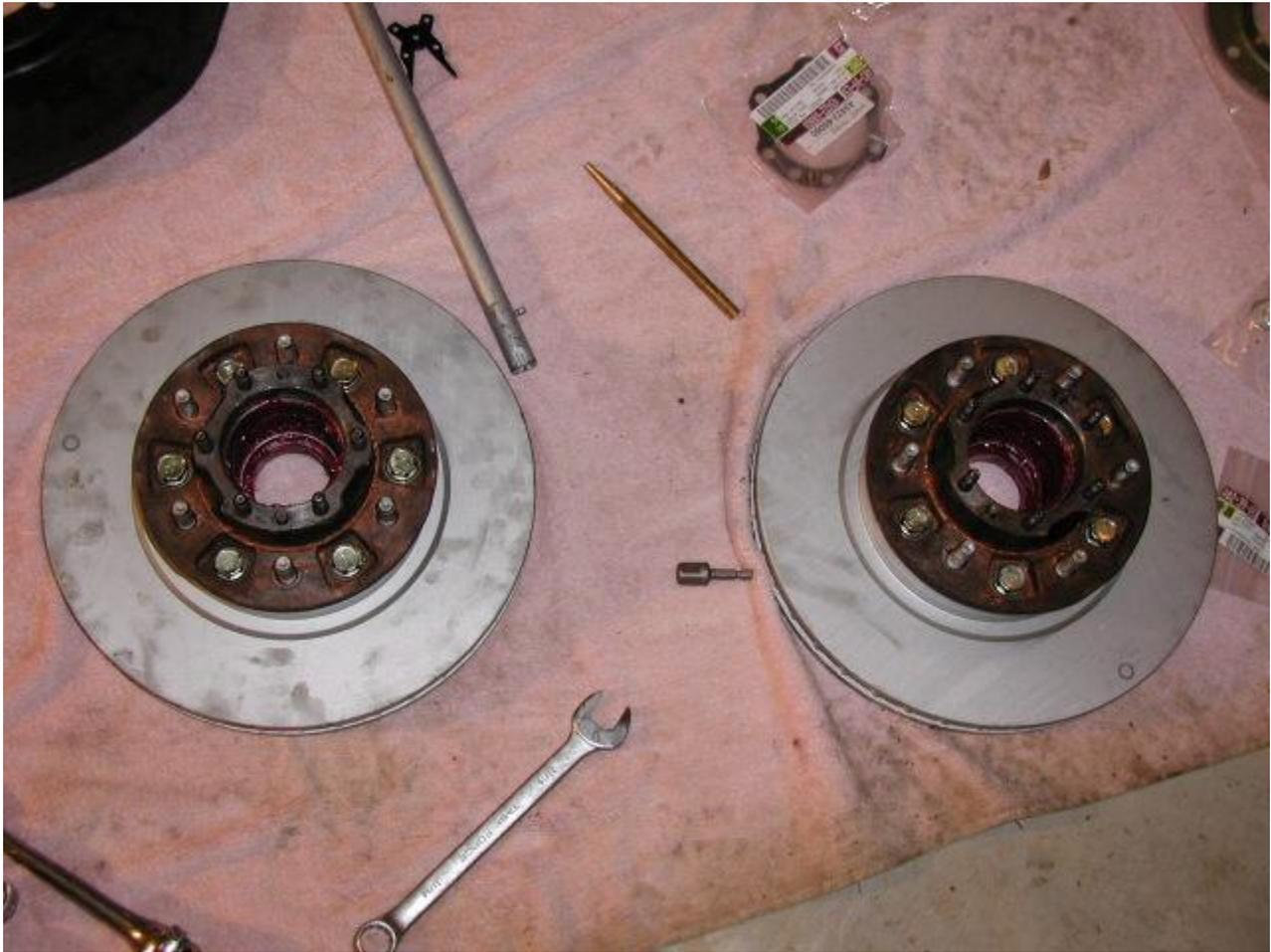
Place the axle hub / disc assy onto the spindle (hub side out)
