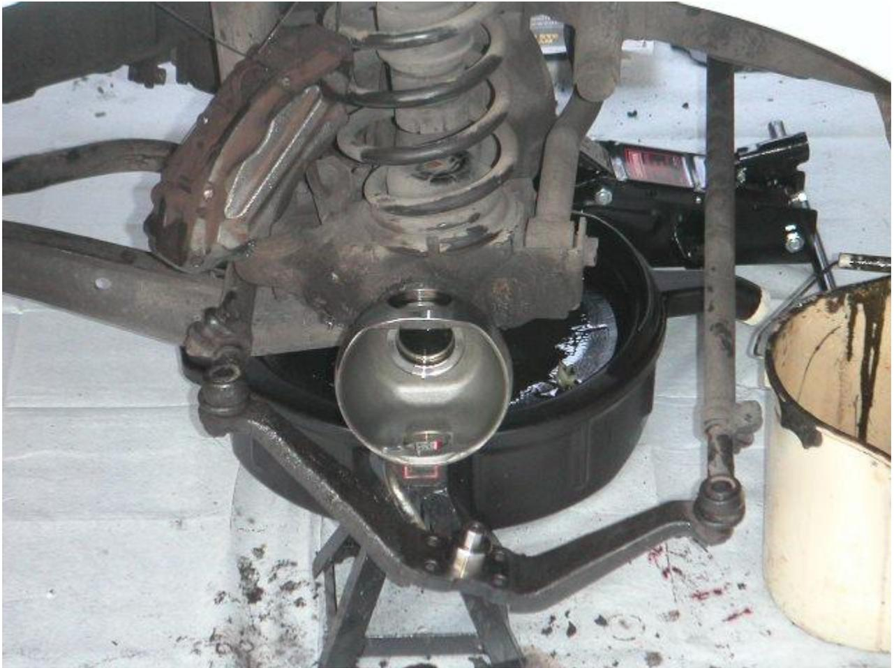
Pic below is a good view of the index ring inside the axle tube:
