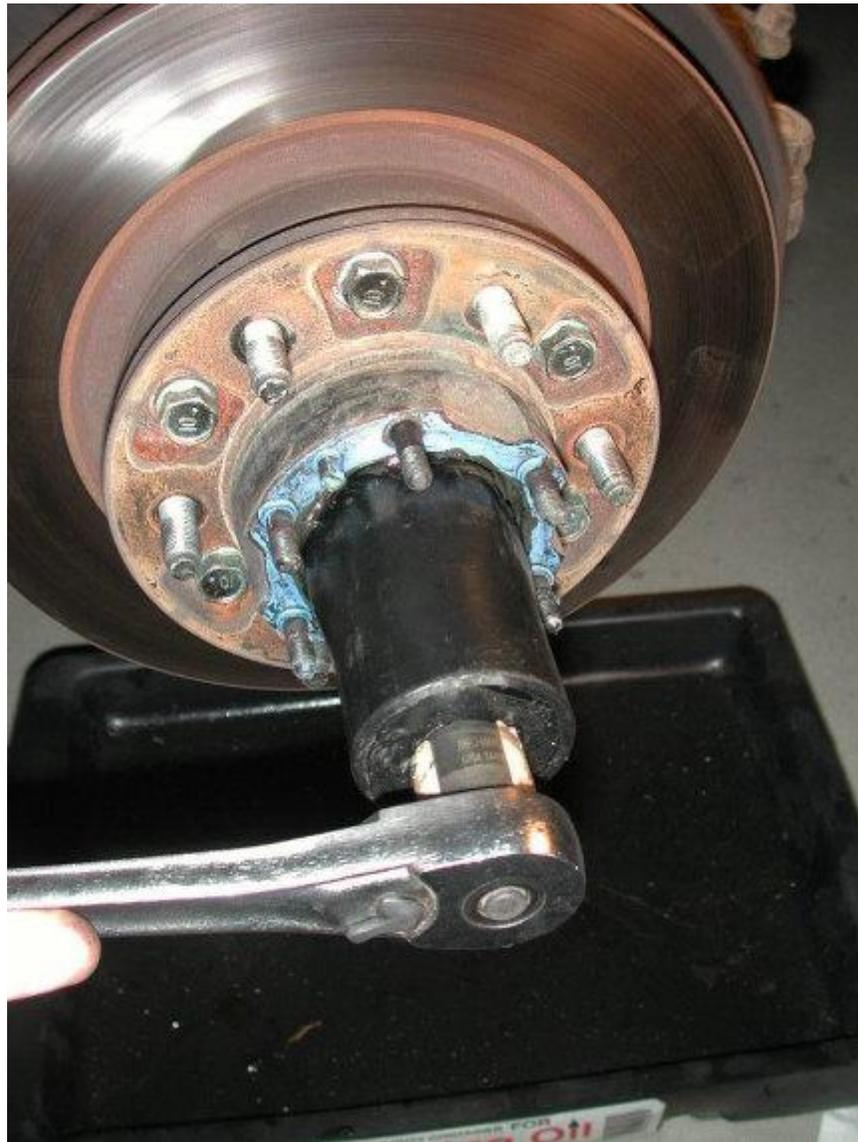
Using the **54MM** Hub Socket, remove the adjusting nut (Used later for preload)
