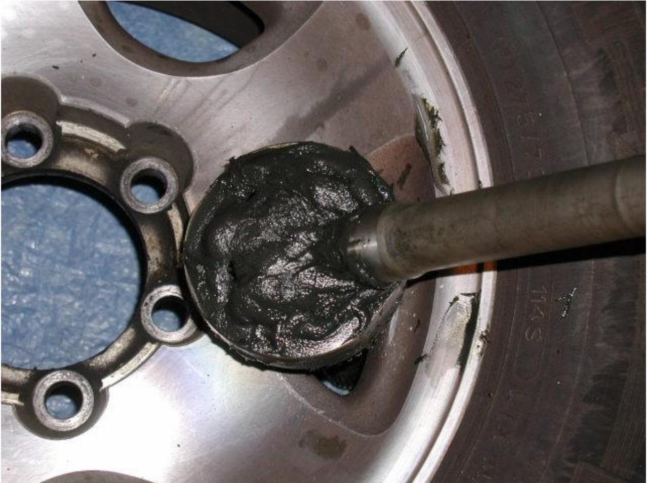
Wipe a light coating of grease over the length of the axle to reduce friction while feeding axle past oil seal
