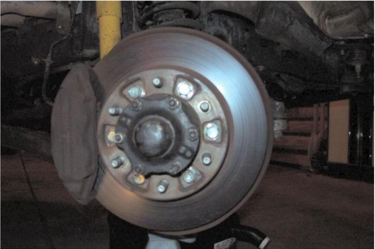
Brake Caliper removed and then cone washers nuts removed from the drive plate. Remove C-Clip
