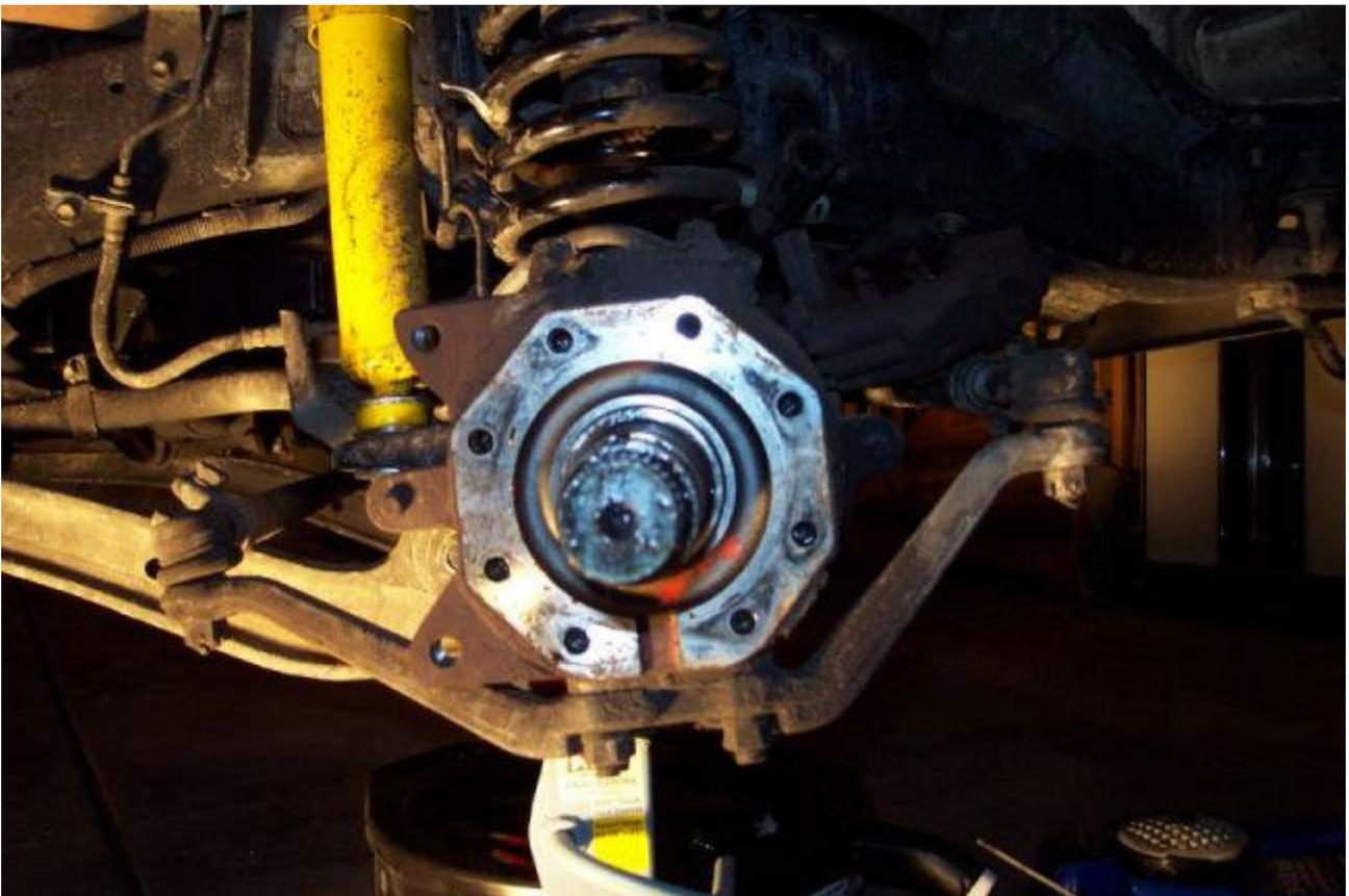
Remove the oil seal set on the back of the knuckle.
