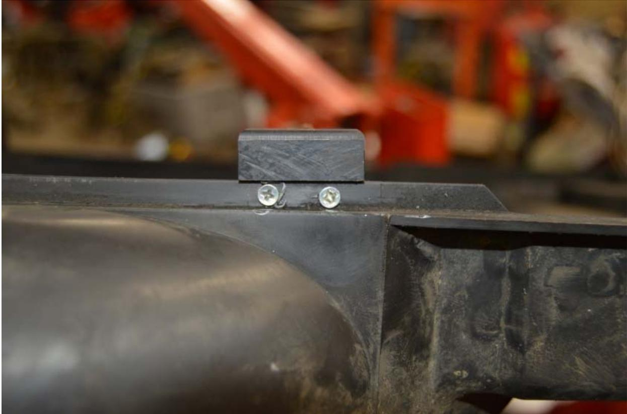
6. Using a drill drum sander or Dremel tool sand the shroud along the front edge of the guard toward the casting marks.
