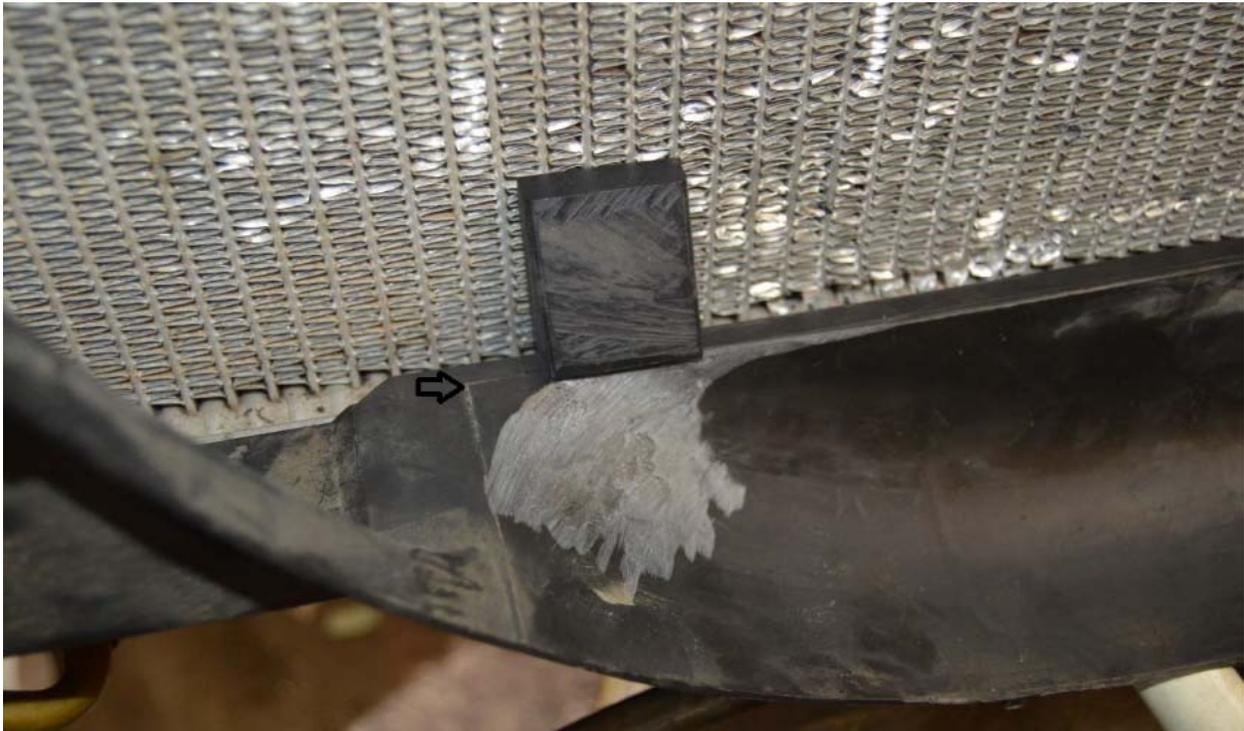
3. Using the 5/64" drill bit drill two holes from under the shroud lip into the guard.
