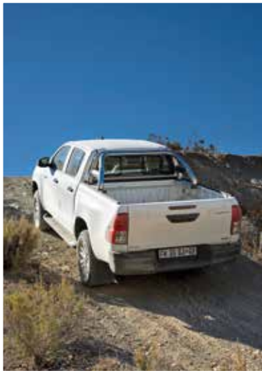
TRACTION. The test was to idle up this steep incline with pressures of up to 2.2 bar. Interestingly enough, all the tyres passed the test, proving that most AT tyres have enough grip and that the differences lie somewhere else.
