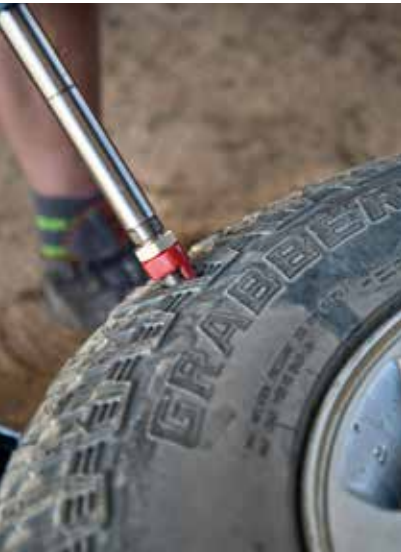
TAKING A STAB. With a lot of the results being quite similar for a lot of tyres, we knew that the dreaded shoulder-puncture test was going to end up making a huge difference in the final score, which it undoubtedly did.
