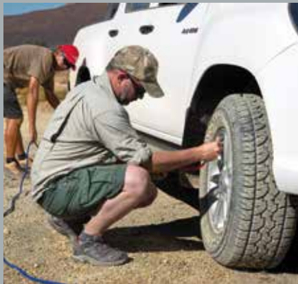
UNDER PRESSURE (top). Tyre pressures are critical for performance, as well as to make sure all the tyres competed on a level playing field. All distances were also meticulously measured after each run (below).
