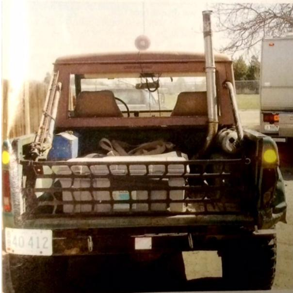
from the beginning. In keeping with that spirit I decided it needed an exhaust with attitude. I ran flexible 3" exhaust tubing straight off the header pipe up through the floor behind the bulkhead to a solid pipe about three feet tall clamped to the back of the cobbled together half cab. A rain cap like you might find on a bulldozer finishes it off. It is not a stealth vehicle. It does, in fact, sound something like a bulldozer.
