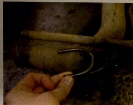
vent lines. The tanks are vented through the caps. Everybody, I hope, knows you don't go welding on gas tanks. However, once the filler necks are removed from the vehicle I have no problem welding on the filler necks. I welded 1/4" nipples down low on each of the filler necks in such a fashion as to direct the fuel being returned back into the tanks.
