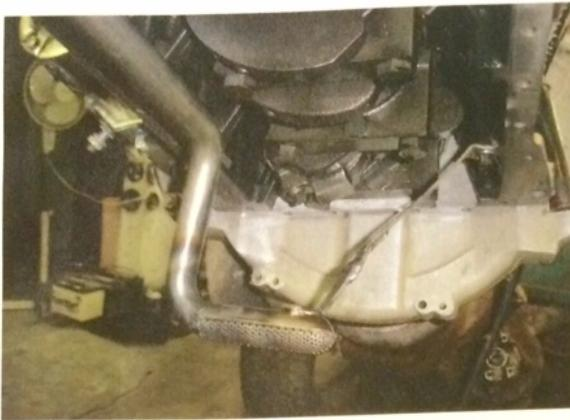
with a slight modification to the oil pickup tube solves this problem while losing only a small amount of its oil capacity.
