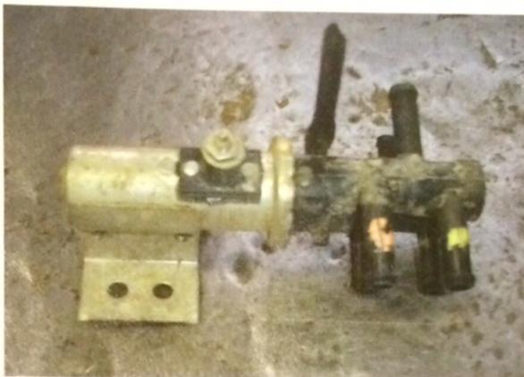
electric six port valve. Universal six port electric valves are, however, easy to come by and reasonably priced. As an added bonus there are three unused terminals on the switch for your fuel gauge that can be wired to switch the valve at the same time you switch the gauge.
