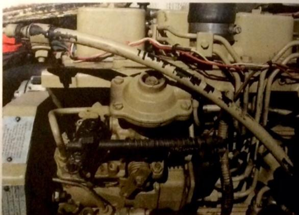
even a small chain out to the linkage on the injector pump. The pump has a built in return spring so no additional return spring is needed.
