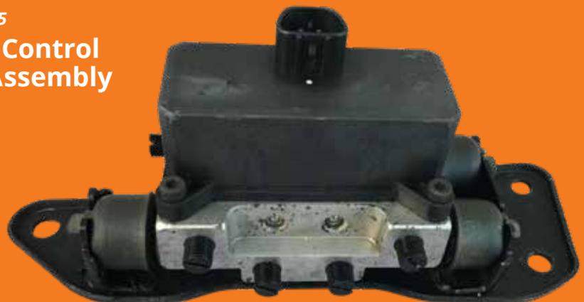
The levelling valves control the fluid between the pump and the gas chambers (globes) located at each wheel.
