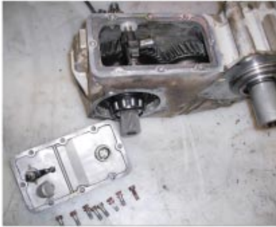
Removal of the shifter cover.
