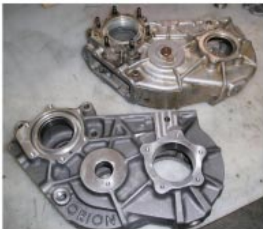
Comparison of the Cast Iron Orion vs. the Stock aluminum case.
