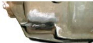
Grinding required on an SM420 case for shifter linkage clearance
