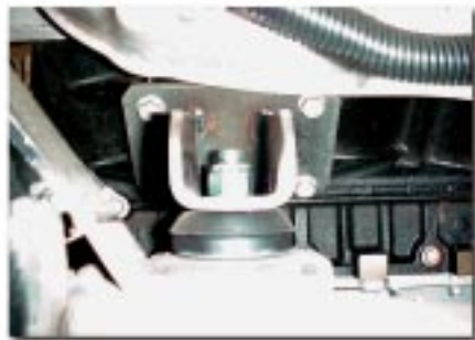
LS1 mount P/N 713088 installed
