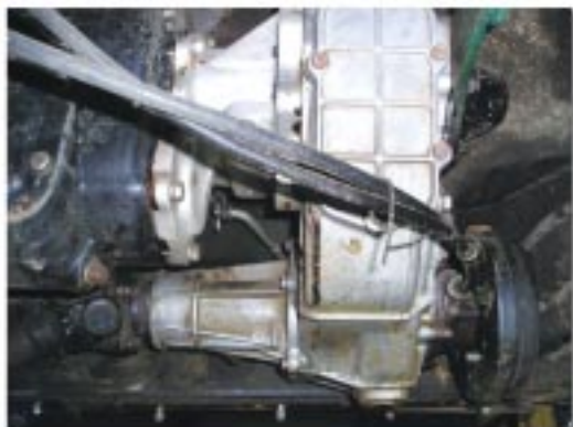
Stock T/C coupled to a SM420 still in the vehicle.
