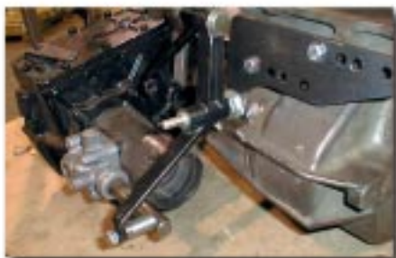
SM420 transfer case shifter bracket
