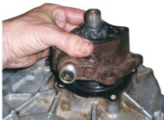
Removal of the stock rear housing
