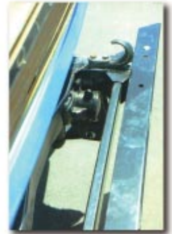
Saginaw steering installed on an FJ55.
