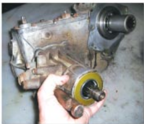
Removal of the stock front housing
