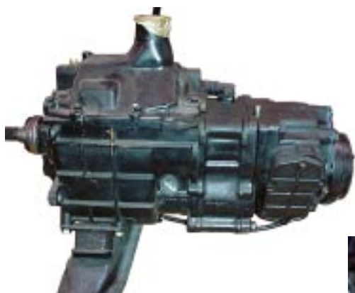
These photos are of an imported Land Cruiser 5 speed. The transmission was coupled to a cast iron, early style transfer case. The linkage used is basically the same as found on U.S. vehicles.
