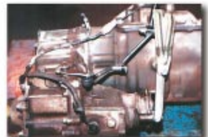
Split transfer case linkage
