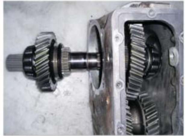
Removal of the rear output shaft
