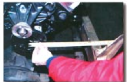
Engine placement offset toward driver's side
