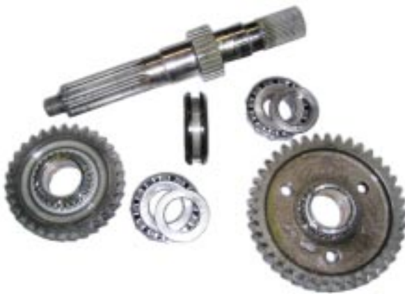
Output shaft assembly.
