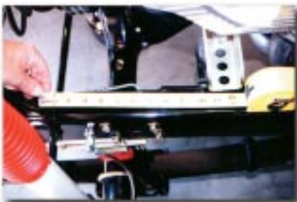
Measuring from the rear of the shock tower to determine the "L" bracket location
