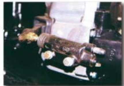
Slave cylinder installed on P/N 712532 bhsg.
