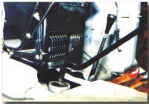
The floor shifter modified to provide heater clearance
