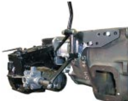
SM465 transfer case shifter bracket
