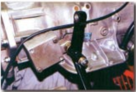
TH400 transfer case shifter bracket
