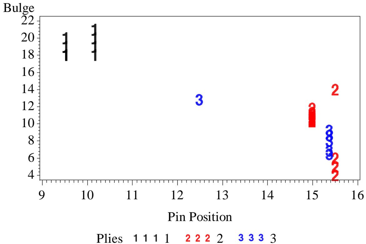
Figure 6.6 Bulge Width Versus Plunger Position and Number of Plies
