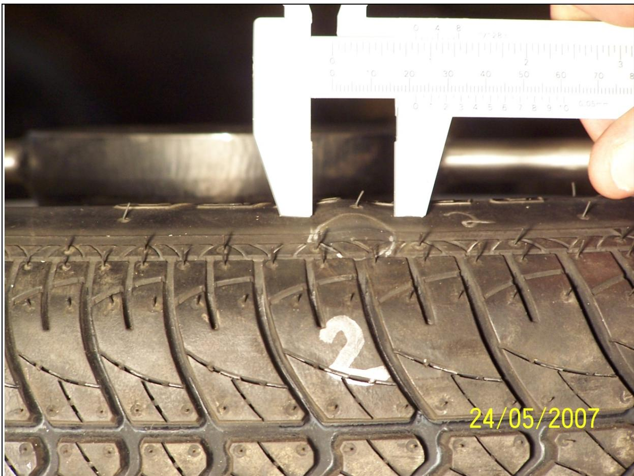
**Figure 6.3 Sidewall Bulge Measurement**
