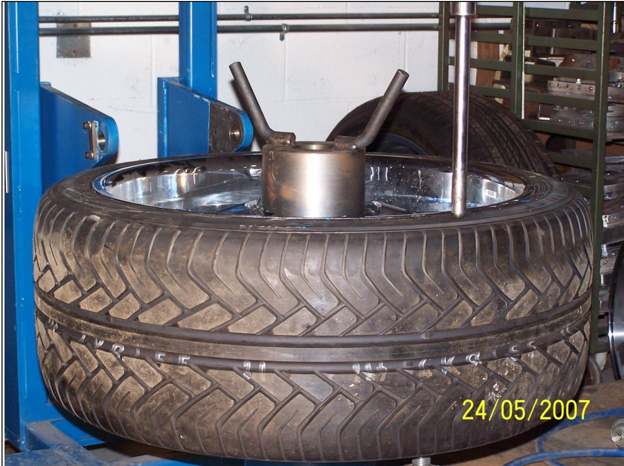
**Figure 6.1 Bead Unseat Fixture with Arm Removed**
