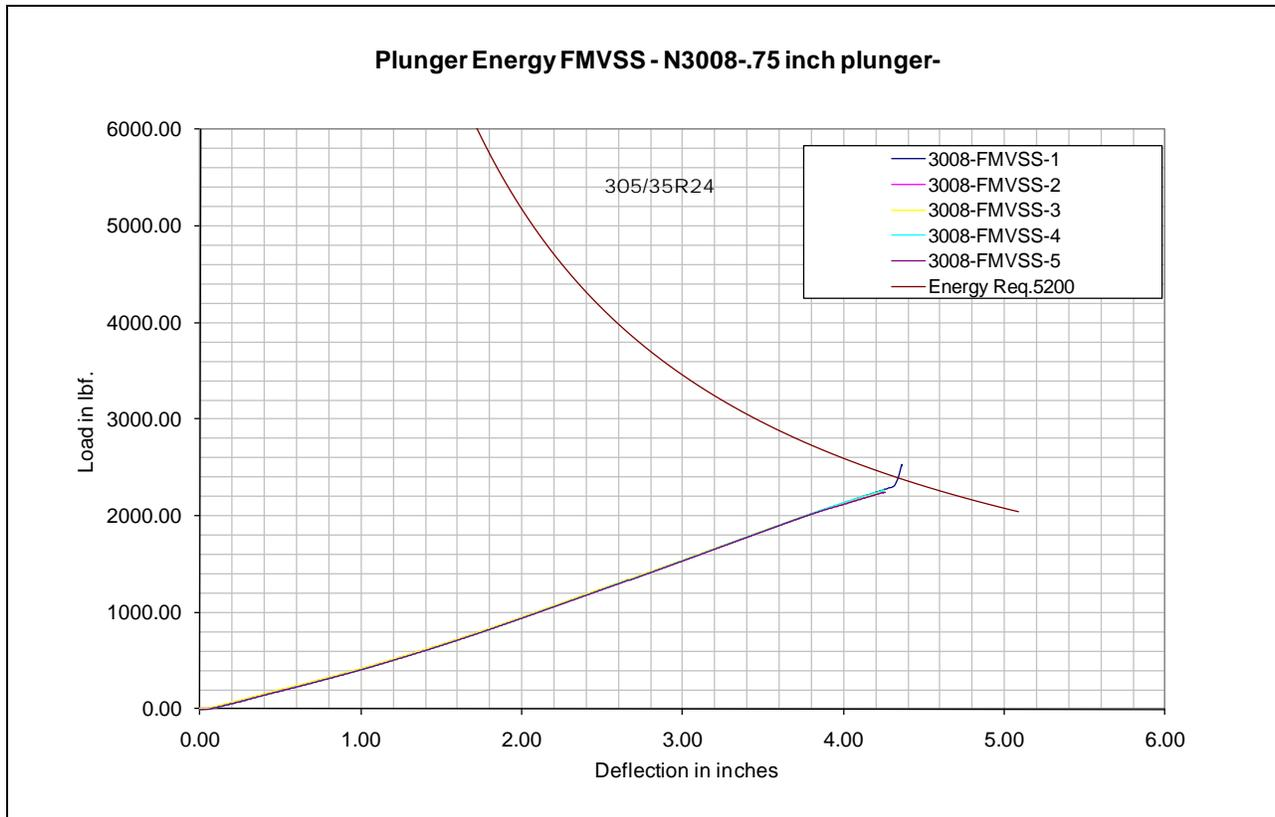
**Plunger Energy ASTM - N3008-.75 inch plunger-**
