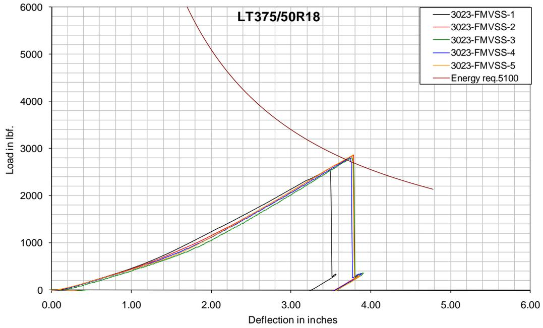
**Plunger Energy FMVSS - N3044-.75 inch plunger-32psi**
