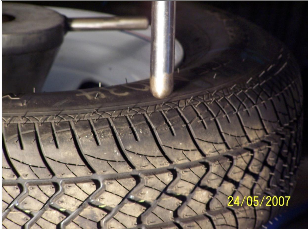
**Figure 6.2 Plunger Placement**
