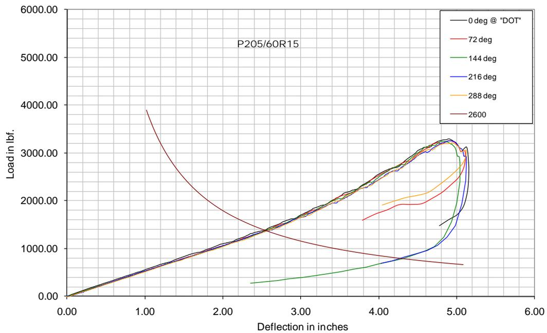
**Plunger Energy ASTM - N3041-.75 inch plunger-26psi**
