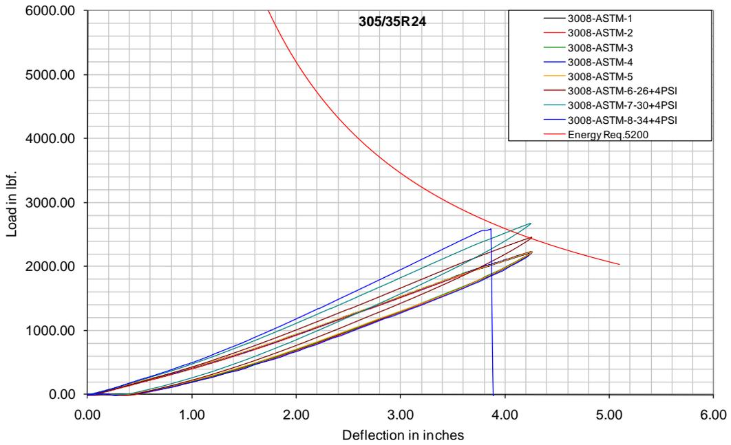
**Plunger Energy FMVSS - N3028-.75 inch plunger-26psi**
