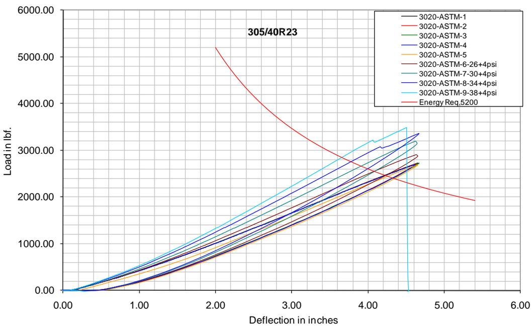
**Plunger Energy FMVSS - N3023-.75 inch plunger-50psi**
