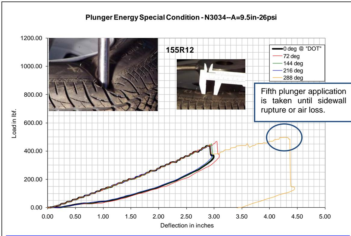
**Figure 6.4 Load-Deflection Curve**
