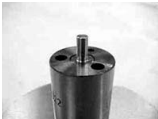
[Nozzle needle with protrusion]
